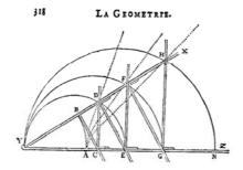
*Figure 9.* Descartes' construction of a curve with the help of an instrument made up of several rules hinged together. Descartes argued that curves described by several successive motions or continuous motion of instruments may yield exact knowledge of the resulting curve (Dover edition of *La Géométrie*, 1954, p. 46).
